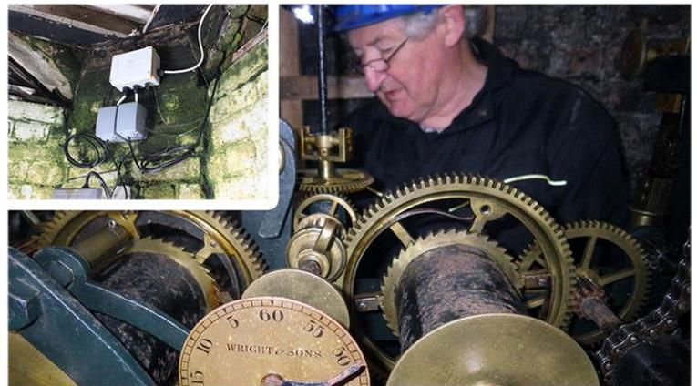
We were quite surprised and shocked to see the interior in such a poor state. However, examination of the striking train shows it is intact and it would be possible to restore the mechanism to bell striking operation.
